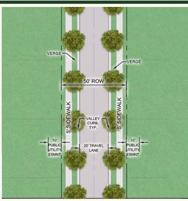
FIGURE 5.3 A1 **Typical 50' ROW Local Street Type 2 Plan Street Tree - within verge**
