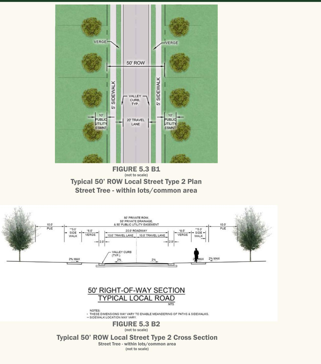
I. Type 2 Local Streets shall be designed and constructed to handle light neighborhood traffic volumes while safely accommodating automobile, bicycle, and pedestrian traffic. II. Type 2 Local Streets are generally two-lane undivided roadways with sidewalks along both sides of the travel lanes. Medians are usually only introduced where the local street intersects a collector or parkway.
