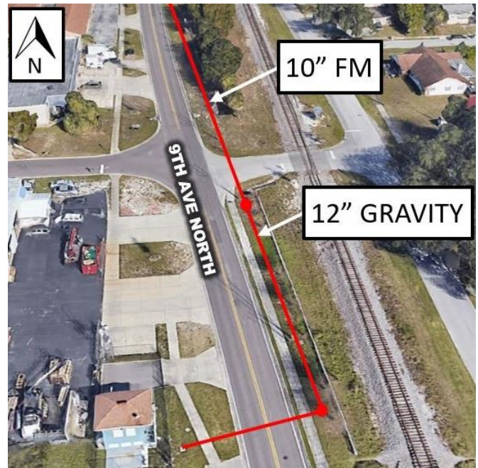
Forcemain Replacement to Main Lift Station
