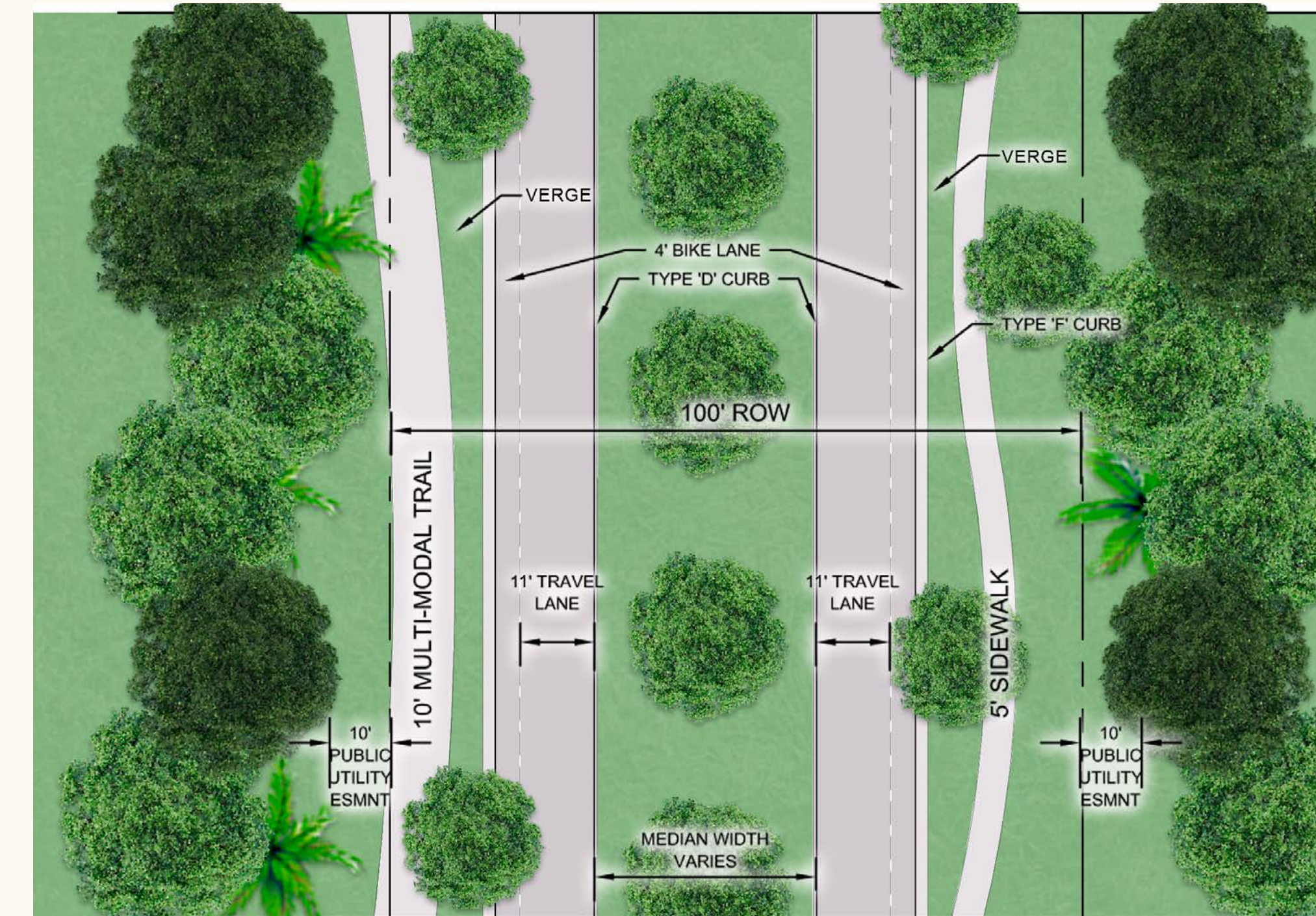
FIGURE 5.1 B1 (not to scale) Typical 100' ROW Collector Road Plan Street Tree - In median and open space
