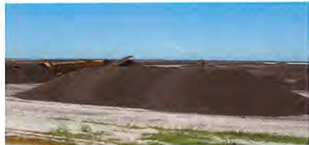
At our Central Valley Compost facility, Synagro utilizes a mobile chip and grind operation for inbound feedstock size reduction.
