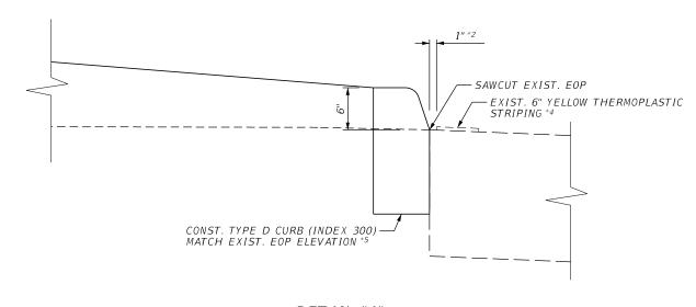
DETAIL "A" N.T.S. CURB PLACEMENT DETAIL
