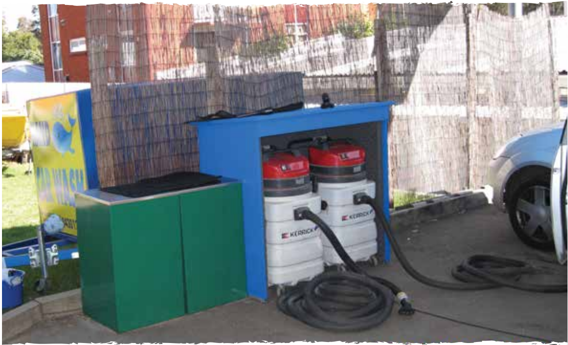
Enclosed noise sources at car cleaning station near residences. Photo: Pittwater Council
