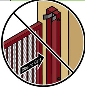
**DO NOT** use a gate catch post. Because the coasting distance may vary due to changes in temperature, it is **NOT** recommended to install a catch post in front of the gate's path. To do so will cause the gate to hit the post in certain instances.
