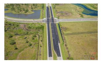
also included maintenance of traffic (MOT), erosion control, earthwork with two pond liners, over 16,000 LF of storm drainage, subgrade, base, asphalt, curb and gutter, landscaping, signing, pavement markings and two new signalized intersections at SR 681 and Laurel Road.
