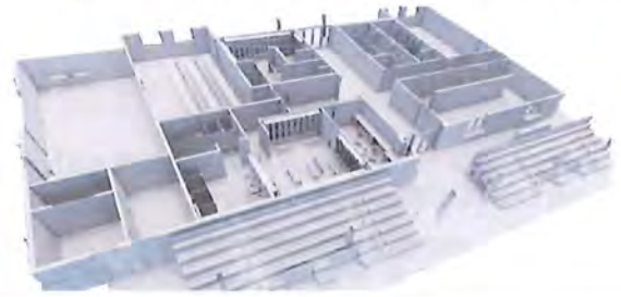
3D computer generated model illustrating used to explore areas of potential conflict.
