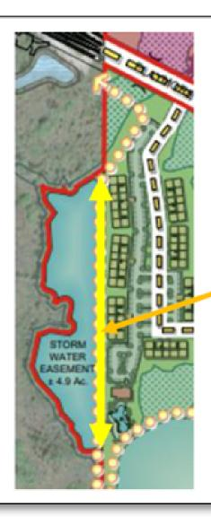
Periphery Height Setback Modification Along Stormwater Management Easement Area
