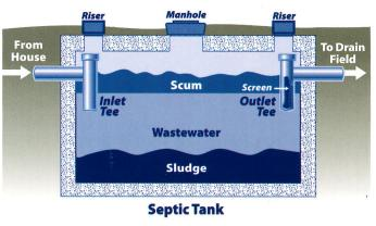
leaving the tank and traveling into the drainfield area. Screens are also recommended to keep solids from entering the drain field. The wastewater exits the septic tank and is discharged into the drain field for further treatment by the soil.
